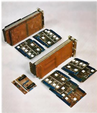
1969 Airborne Command & Control station. Multilayer boards / rack-mounted modular ATR boxes, micro-processor control. Automated manufacture. State of the art electronics.
