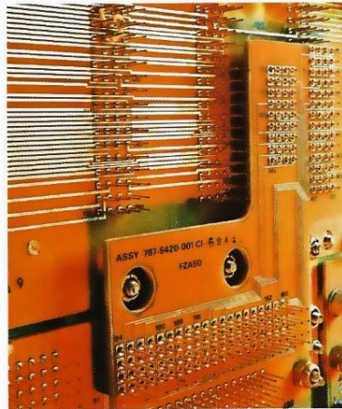
1969 Airborne Command & Control station. Multilayer boards / rack-mounted modular ATR boxes, micro-processor control. Automated manufacture. State of the art electronics.
